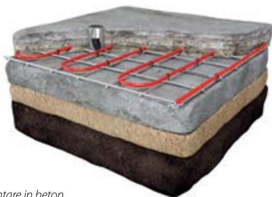
Montare in beton
